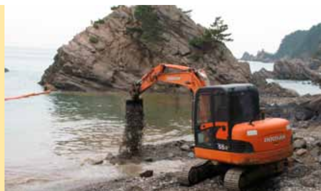
An excavator shifting sand to accelerate natural cleaning of oiled pebbles following the Hebei Spirit incident.
