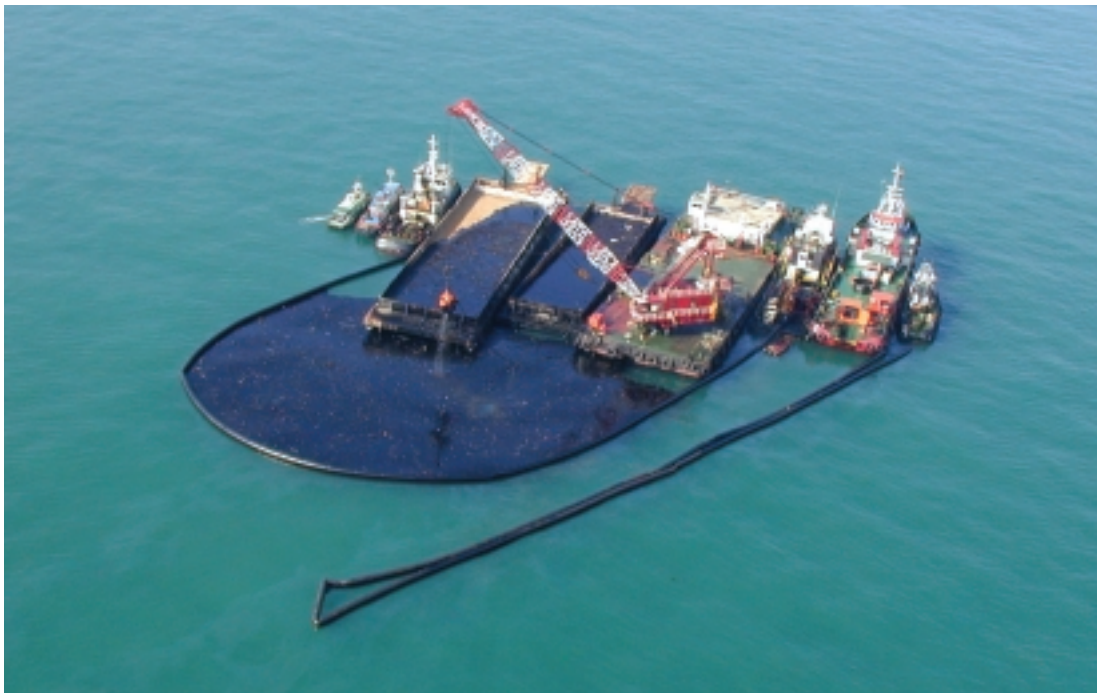
Natuna Sea: containment and recovery of weathered oil at sea
