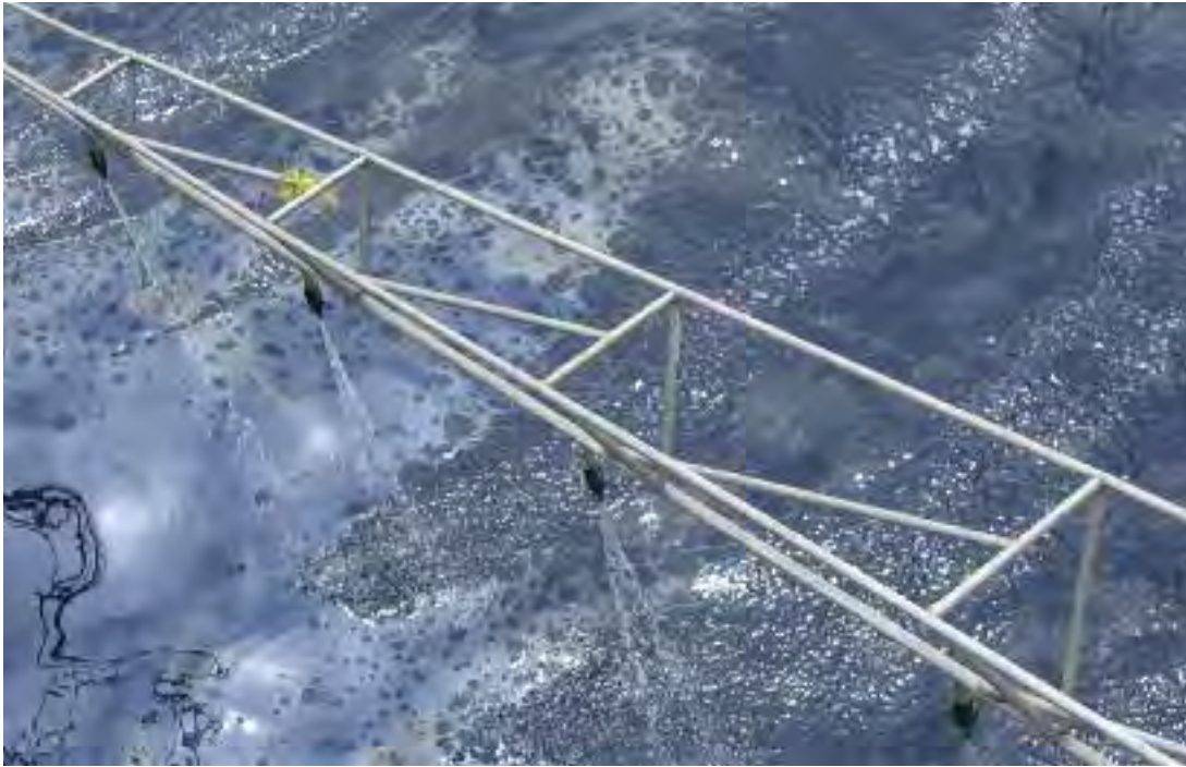
Solar 1: Application of chemical dispersant from a ship-mounted spray arm
